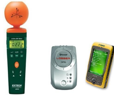
Fig 2. EXTECH Instruments RF EMF Strength Meter and GPS with data logger used in measurements
