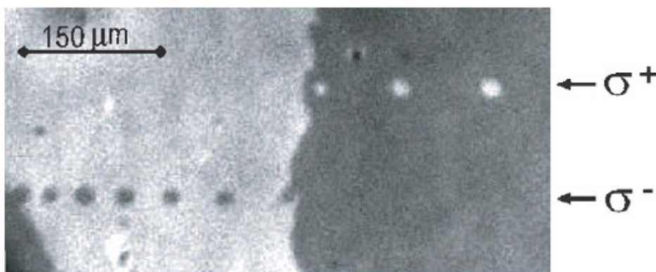
FIG.3. All-optical magnetization reversal using the inverse Faraday effect [10].
