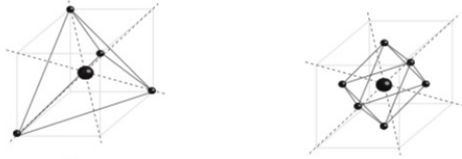
Fig 5. Tetrahedral and octahedral sites, showing how each has cubic symmetry
