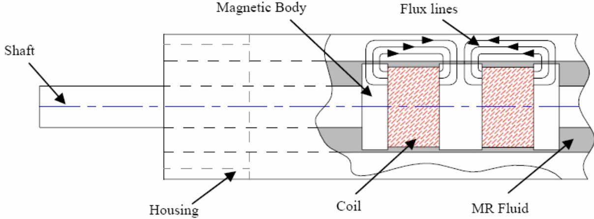
Fig. 1. Schematic of the double-shafted MR damper
