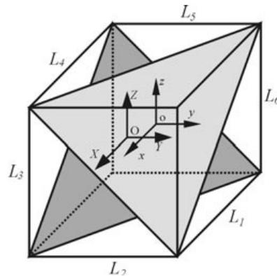
Fig. 2 Cubic configuration of a Stewart platform
