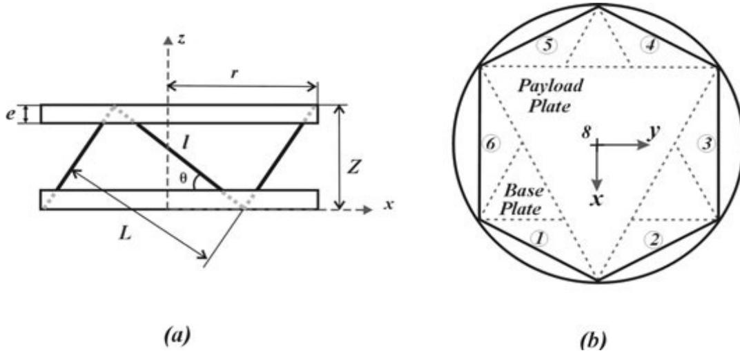
Fig. 3. Schematic drawing of Stewart platform; (a) side section, (b) top view [9]
