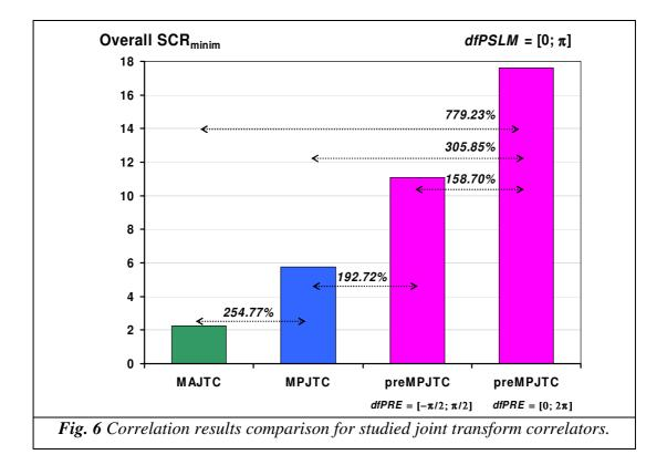
The preprocessed modified joint transform correlator has different behaviours in relation with the amplitude premodulation domains. In the first case,  $dfPRE=[-\pi/2;\pi/2]$ , it has the same behaviour as the other two correlators with a increase of detection efficiency (*SCR* coefficient). In the second case,  $dfPRE=[0;2\pi]$ , the detection efficiency is relative high only for nonzero background images and is smaller in the null background level images.
