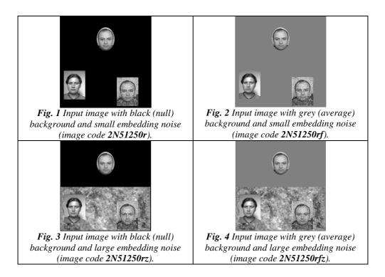
The embedding noise has a poor effect on detection efficiency (*SCR* coefficient) for all three modified joint transform correlators, thus these correlators are very robust to any embedding noise.
