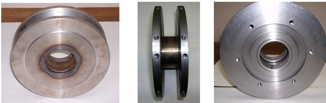
**Fig. 4.** Stages of L2 execution. Left: the spool after welding, with the welding belts at the inner sides of the flanges. Middle: the flanges, with holes for fastening a soft iron cover. Right: the spool, after adding the polar pieces, facing, and boring.
