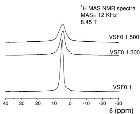
Fig. 1. <sup>1</sup>H MAS NMR Spectra of VSF0.1, xerogel and thermal treated at 300 and 500°C
