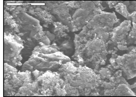
**Figure 3.** SEM image of obtained soft carbon
