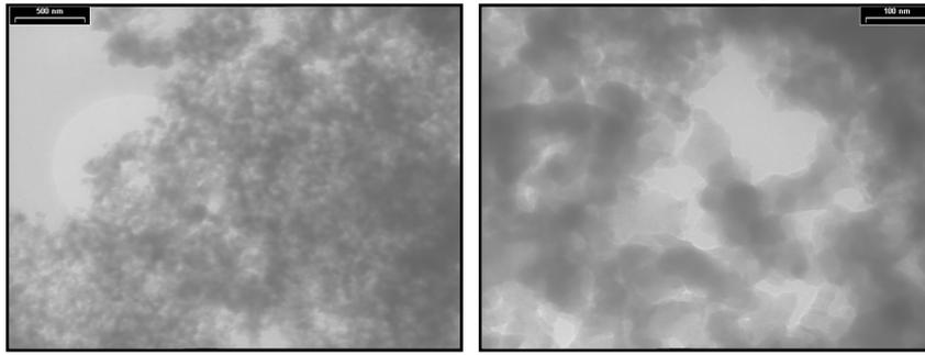
*Figure 6. TEM images of hard carbon at different scales*
