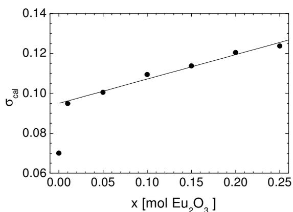
*Fig. 1 Compositional dependence of the Poisson's ratio for the xEu<sub>2</sub>O<sub>3</sub>(1-x)[3Bi<sub>2</sub>O<sub>3</sub>·PbO] glass system.*
