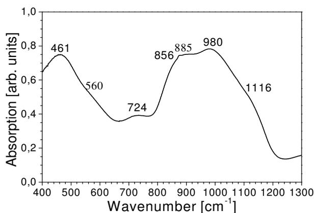
Fig. 2 IR spectrum of the  $3\text{Bi}_2\text{O}_3\cdot\text{PbO}$  glass matrix
