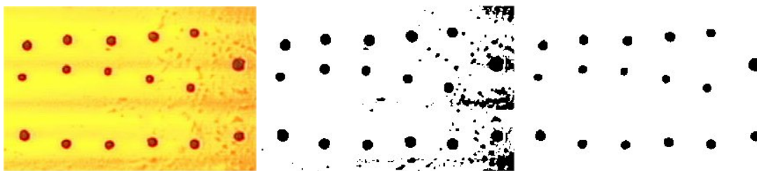
Fig. 2. Defect enhancing using simple filters.
